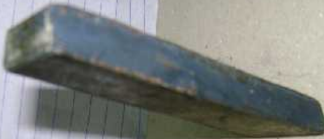
Copper piece placed at cooling tower (Tin Coated)
